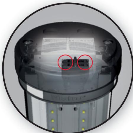
Two opening switches allow the light source and the battery to be switched off automatically when the luminary flange is open.
