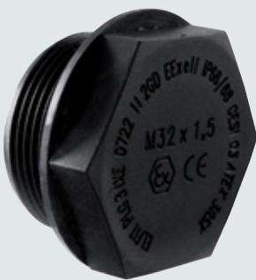
PLG series polyamide plugs are used to close the unused entries in case of Ex e/Ex i certified enclosures (for intrinsically safe circuits, plugs can be supplied blue coloured).
