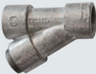
Sealing fittings prevent the passage of gas, vapors or flames through pipes system. EYS series vertical fittings are available in two different dimensions: the first up to 1"; the second up to 3" with an additional lateral opening for easy insertion of glass-fiber. EZS series are used for both vertical and horizontal mounting.
