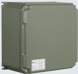
AQ../AR.. Series are used to house Ex e and Ex i terminals. Maximum number of terminals changes on the base of terminals section, enclosure operating temperature and required temperature class. They are ideally suited for chemical agents environments. Sea water corrosion resistance and extremes of low and high temperatures.
