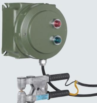
Control and discharge system for electrostatic charges suitable for road tankers, rail tankers and any movable tanker for dangerous items, ready for one/two double circuit clamps PTA ISE0-2. System is complete with arrest/consensus optical warning and changeover contact free from output voltage. The solution to control the discharge of static charges driving it through a dedicated and safe path, safe becauseExplosion proof.
